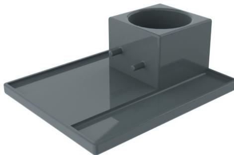
The Plastic base will be acquired by the assembly worker and placed into a simple fixture so that it is ready to receive the remaining parts.
