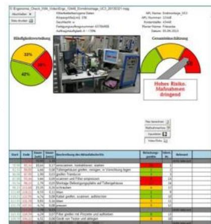
Based on the standard EAWS-From V1.3.3 which was designed and used by the automotive industry we evaluate the movements registered and identified on the video and label them. The result of the
