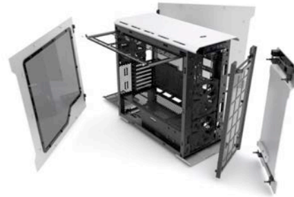
Typical Desk Computer Housing Stamped Metal and Injection Molded Plastic
