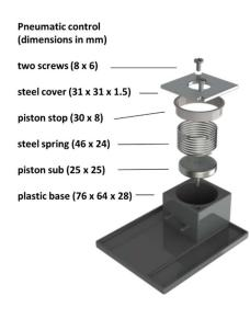
This process can be illustrated using a product which is an example frequently used during initial DFMA training with BDI. This product is a simple piston mechanism used in printers during the middle 20<sup>th</sup> century. The picture of this product is seen at left.
