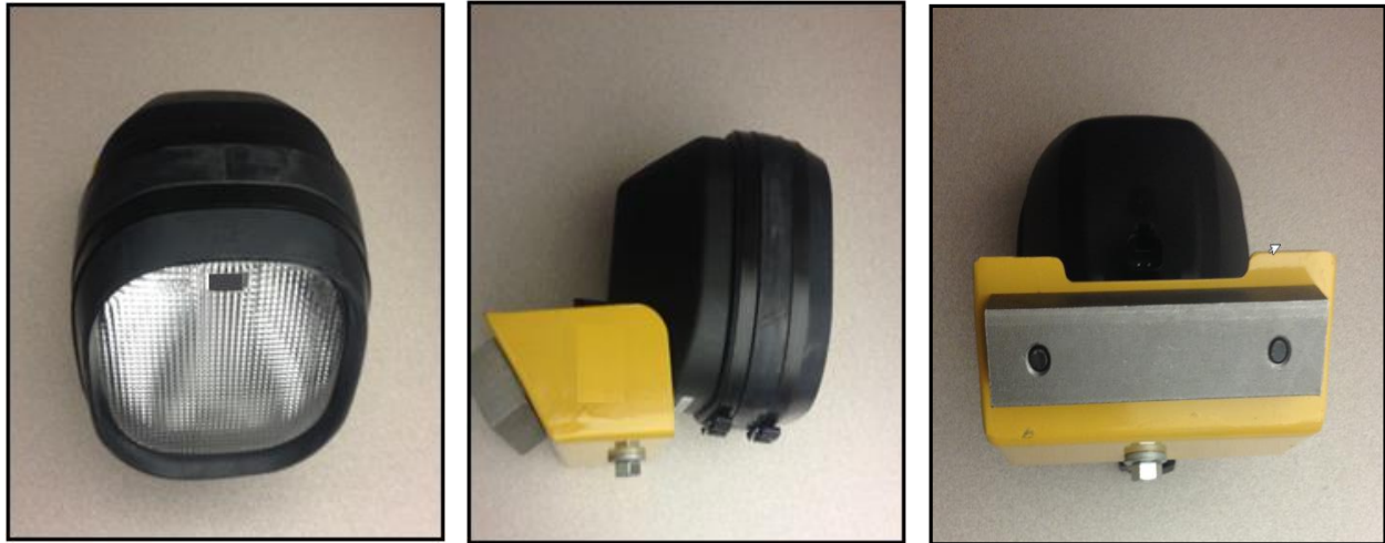
Figure 4 Rear lamp assembly - cost reduced redesign.
