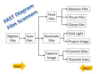
Data, and Transmit Data are functions that all film scanners must perform. By functionally organizing data, one can see how different designs compare and how a specific company might be evolving their technological solution over time.
