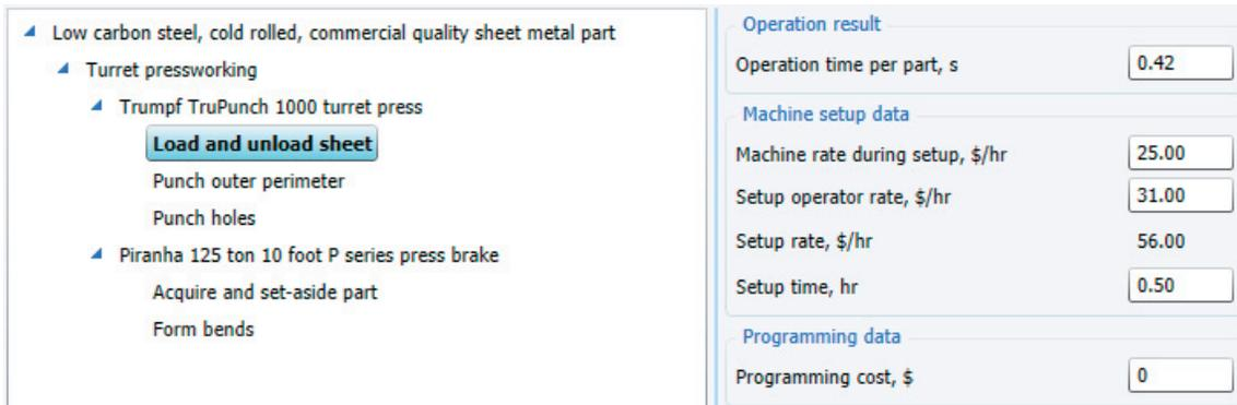
Now we are going to change the sheet metal process type and do a cost comparison of the two processes.
