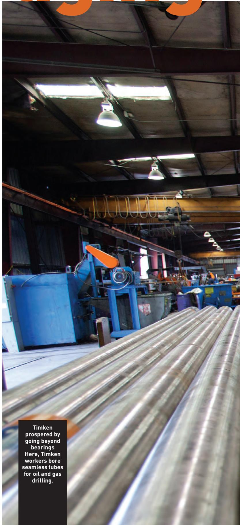
Timken prospered by going beyond bearings. Here, Timken workers bore seamless tubes for oil and gas drilling.
