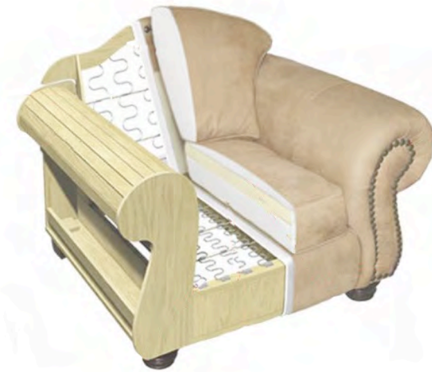
Typical Chair Substructure Cut / Formed Wood, Foam, Fasteners
