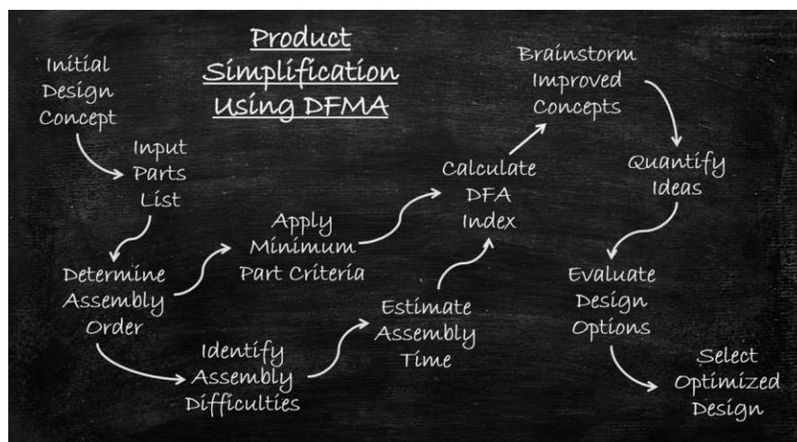
The next step is to organize the parts in the expected order of assembly. List any reorientations of the parts or product while visualizing the assembly of the parts. Additionally, identify any necessary operations, such as: adjustments, securing of parts, tightening, material applications, testing and inspections.
