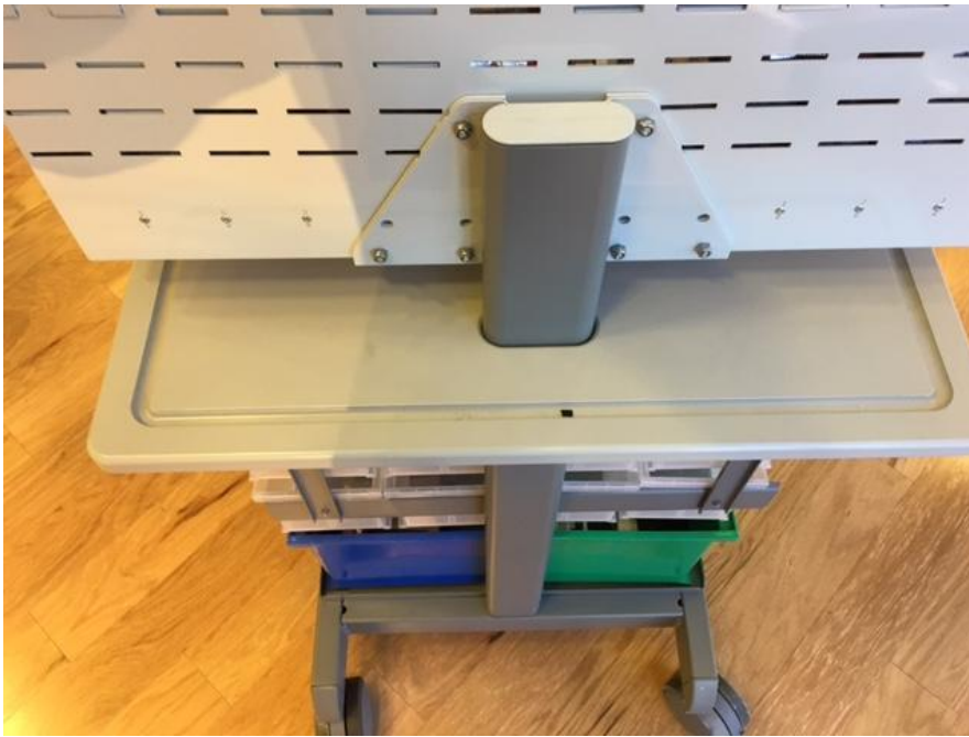
Figure 15 - Original design showing structural steel tubing spine
