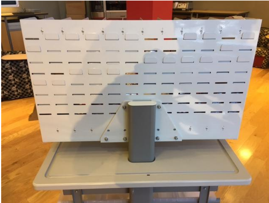
Figure 17 - Original design showing separate brackets to secure top divided compartment to spine - Also shows pop-riveted construction used on vertical dividers.
