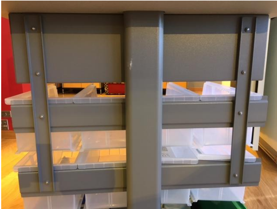
Figure 19 - Original design showing four center bin brackets pop-riveted together and to cart's spine
