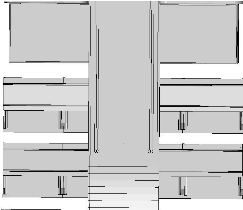
Figure 20 - Redesign showing two center bin brackets welded to cart's spine
