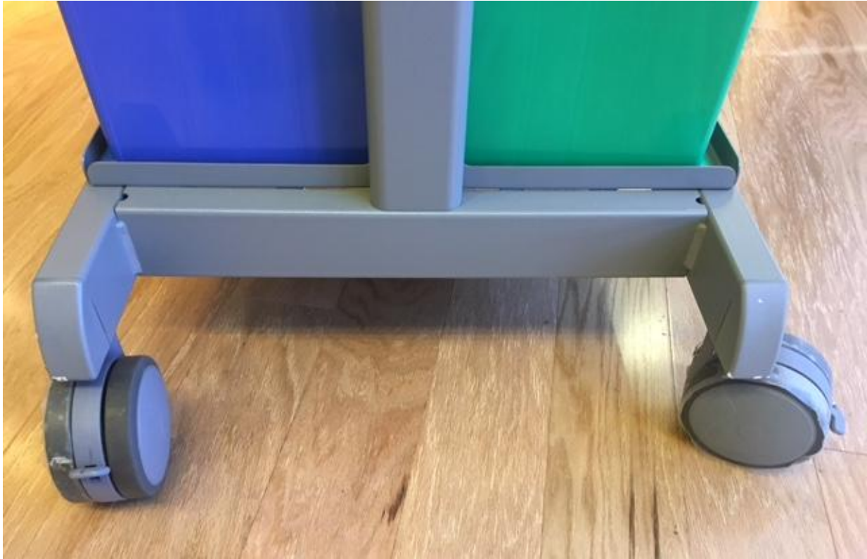
Figure 13 - Original design showing attachment of casters and exposed welds
