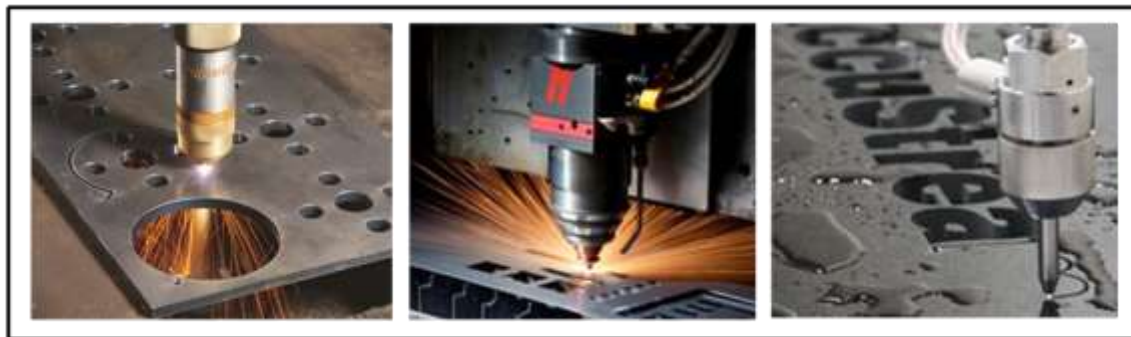
Figure 3. Hypertherm plasma, laser, and waterjet cutting.
