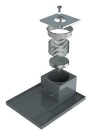
In this tutorial, we will add to this analysis an operation for applying thread locking compound to the two screws that hold the cover in place.
